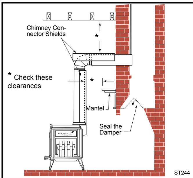
Fig. 7 Chimney connector enters chimney above the fireplace.
