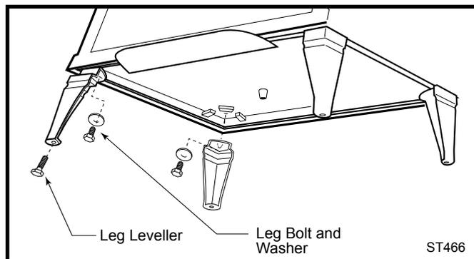
Fig. 26a Attach stove legs and leg levers.
