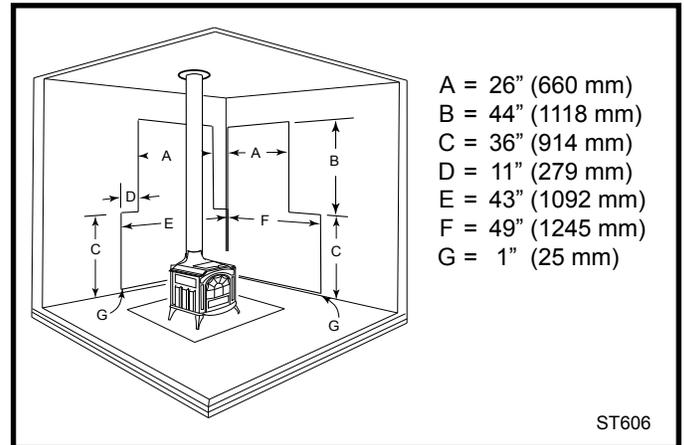
Fig. 20 A top-exit stove with reduced rear and side wall clearances. Note that rear wall shield must extend completely to corner.
