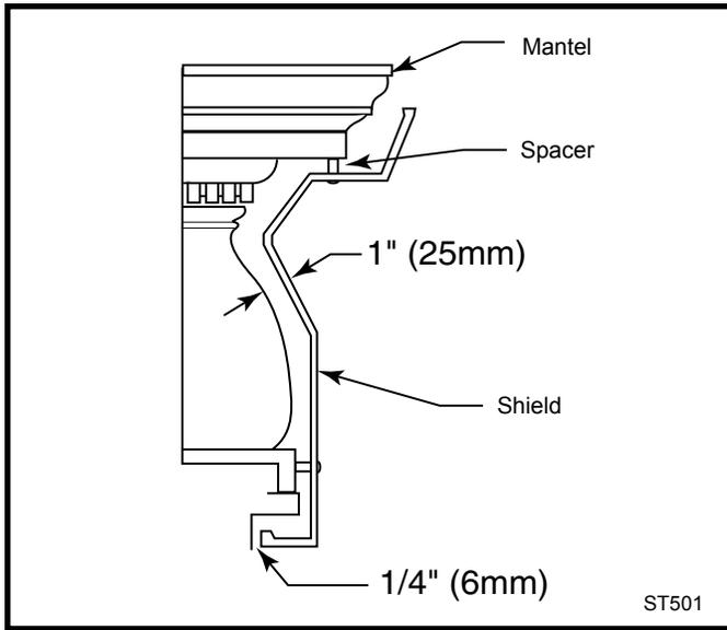
Fig. 14 A custom-formed mantel shield.
