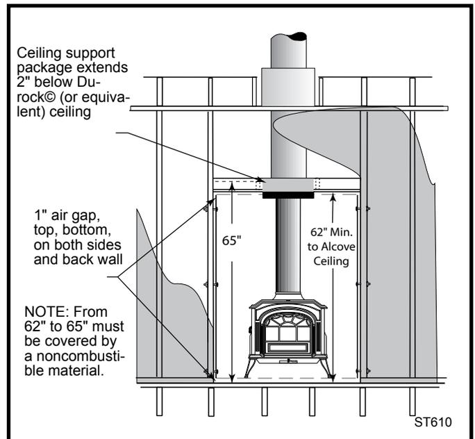
Fig. 26 Front section: 65" minimum clearance to combustibles on front face. Combustible facing may overlap metal studs by only 1". It should not extend below the height of the noncombustible ceiling.
