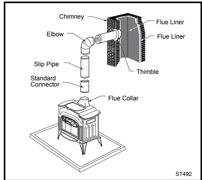
**Fig. 6** Chimney connection is a freestanding installation.
