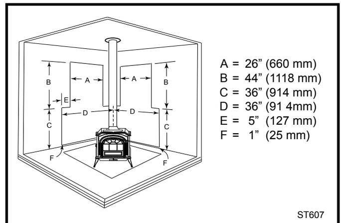
Fig. 21 A top-exit stove with reduced rear and side wall clearance. Wall shields must meet at corner.
